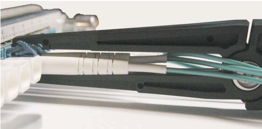
Figure 14: “Skinny Fingers” Gripping a Densely Packed LC Connector
