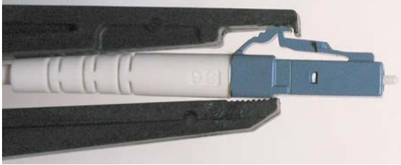
Figure 7: Proper Grip Applied to Dual-Piece Latch
