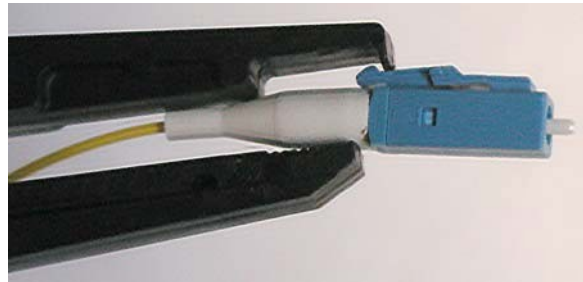
Figure 4: Compressing the Single-Piece Latch for Insertion or Extraction
