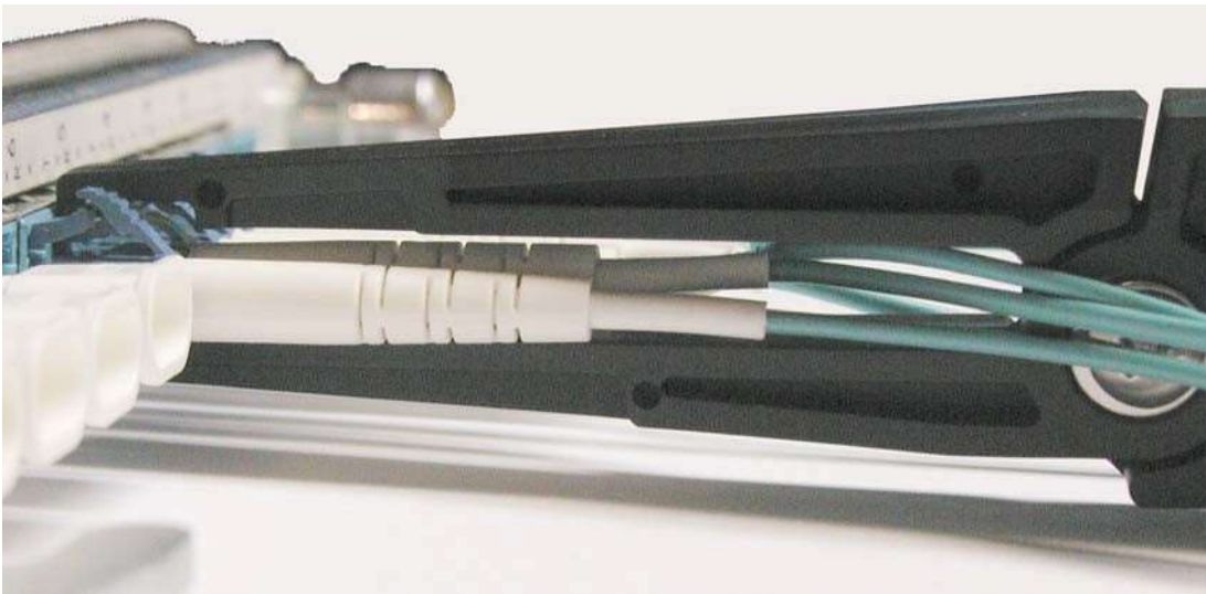
Figure 14: “Skinny Fingers” Gripping a Densely-arrayed LC Connector
