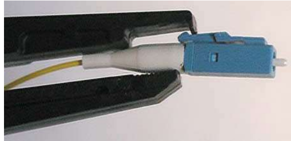
Figure 4: Compressing the Single-Piece Latch for Insertion or Extraction
